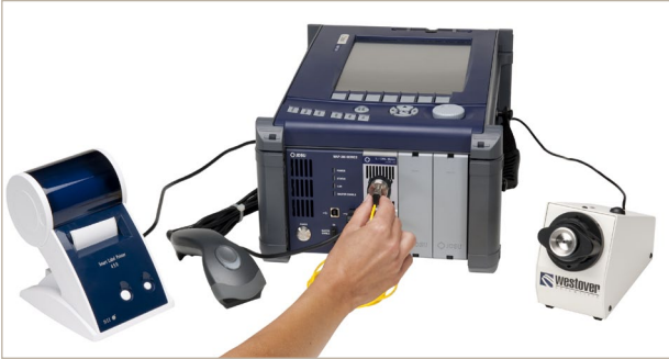
Figure 8: Example using the JDSU FVD to verify the connector end face of the jumper under test
